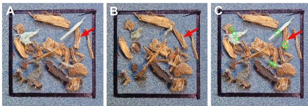
Figure 2. Subsequent images of a compost sample, spread across a 1 cm 2 area. A – before heating, B – after heating, C – algorithm processed.
